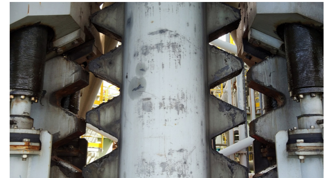
Hydraulic jack-up mounted on a truss type platform leg.
